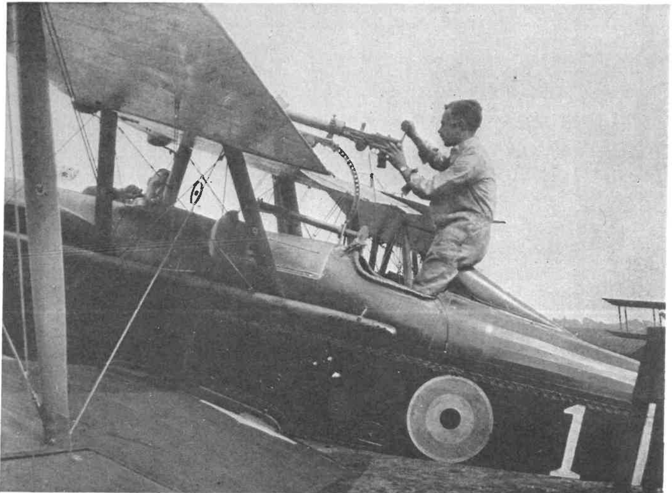
Capt J M Robb (later ACM Sir James) of 92 Squadron adjusting the sights on his SE5A's Lewis gun.
